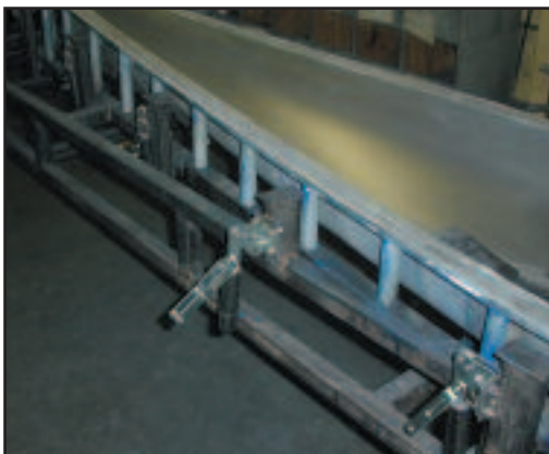
◀ On this kayak mold, the customer uses model 311 with a pipe handle to hold the mold halves together.
