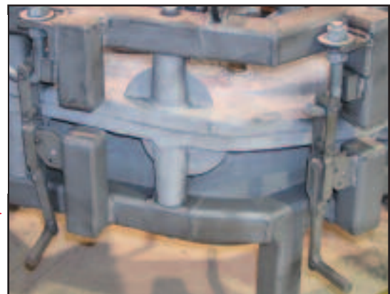
301-22 clamps are used to hold together two mold halves. ▶
